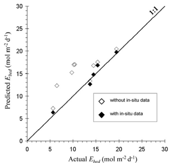
**Figure 11.** Predicted daily benthic PAR ( $E_{bed}$ ) versus actual  $E_{bed}$  at BSC for 16–25 June 2006. Predicted  $E_{bed}$  was modeled using equation (5). Actual  $E_{bed}$  was measured with an underwater PAR sensor. In situ data include  $s$  and  $K_d$  derived from the sensor array (Appendix C).
